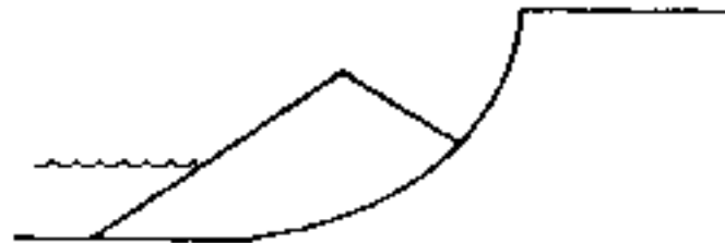
C. Bank may fail because of pressure imbalance.
